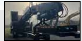
2023 Rotobec Evolution 965 Log Loader S/N: 196302-1-1, Cummins QSB 6.7 Tier 5 Stage V (173 HP), 32'6" Boom Bar, Saw/Pull Through, Hydraulic Optio Carrier Ready Less, Main Valve Option, Dead Heel
